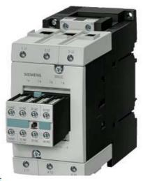
CONTACTOR, AC-3 37 KW/400 V, DC 24 V, 2 NO + 2 NC, 3-POLE, SIZE S3, SCREW CONNECTION
